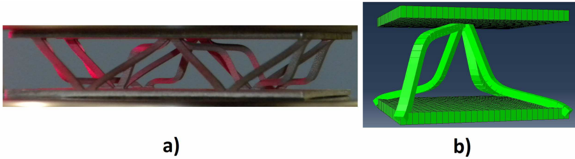
Fig. 1: a) Compression experiments of the pyramidal truss core structures. b) Finite element representation of the unit cell of pyramidal core. (Shell and beam profiles are rendered by Abaqus.)
